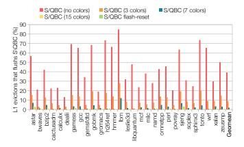
Figure 9: Percent of cache line evictions from L1 that cause a S/QBC flush with, 2, 3, 4 dirty bits (3, 7, 15 colors) and using flash-reset. (lower is better)
