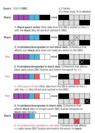
Figure 6: Operation of the S/QBC with red/black dirty bits. Only coherence actions on L1 data that affect dirty data from the current epoch result in flushes of the SBC and a color change.
