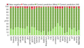
Figure 7: Memory dependency predictor accuracy using dynamic store-distances. Overall, it is able to predict 93.6% of S/QBC accesses correctly.
